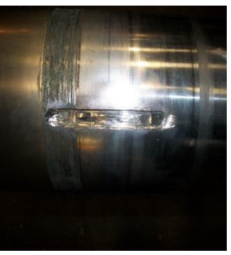
After the keyways were welded complete, the shaft was put on the machine and M/S proceeded to machine the old metal spray off the shaft. This was no easy task being that the shaft wall thick ness was only .200" thick. The metal spray was .095" thick. This being said it was a very delicate process. Metal Surgery took extra precautions by ordering and machining a spare piece to be machined and welded on incase the piece was not salvageable.
