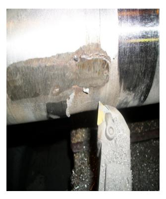
On the right illustrates all the old metal spray removed. The piece was then prepped for metal spray by blasting
